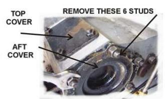
Remove the six nuts holding the round PTO cover and the four nuts holding down the transfer case top cover. Both covers can be stored as they are no longer required. The four nuts and washers for the top cover will be re-used and the four studs are left in place. The six studs that held the aft cover must be removed. A vise-grip can be used for this purpose or two nuts locked together.
