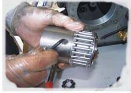
screws on the periphery of the coupling are sitting flush with the outer surface. Remove the hexagon nut from within the cupling.
